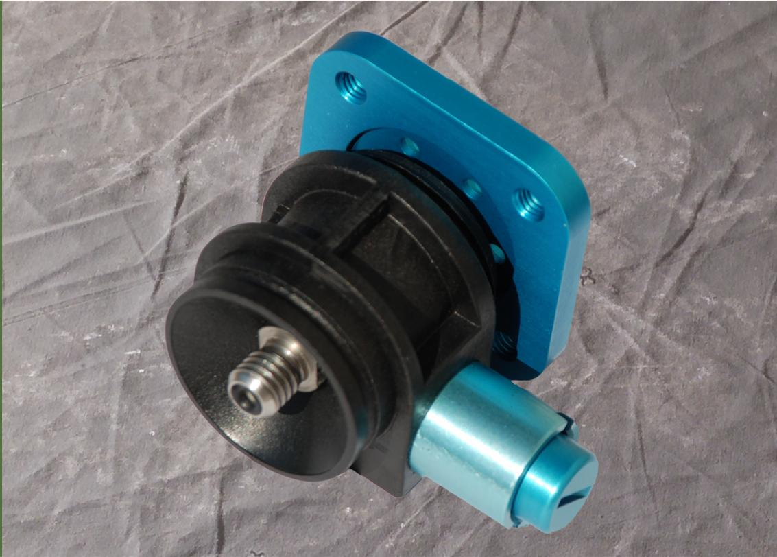
The ALPS Lock Flat Bottom includes a lightweight aluminum plate with a 4 hole pattern for attachment to a 4 bolt pyramid component. This lightweight locking device made of glass reinforced nylon exhibits better wear characteristics than derin or aluminum. The convenient one-way gear allows the user to push in or wind the limb into the socket. A unique feature of this lock is that if foreign material or clothing get caught in the gear, the housing can be removed freeing the pin.
